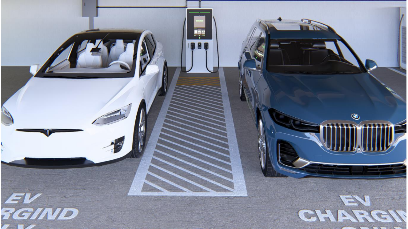
Figure 7-8: Illustration of a dual-port DC fast charger setup showing a centrally located unit serving two adjacent vehicles with cables extending to both sides.
