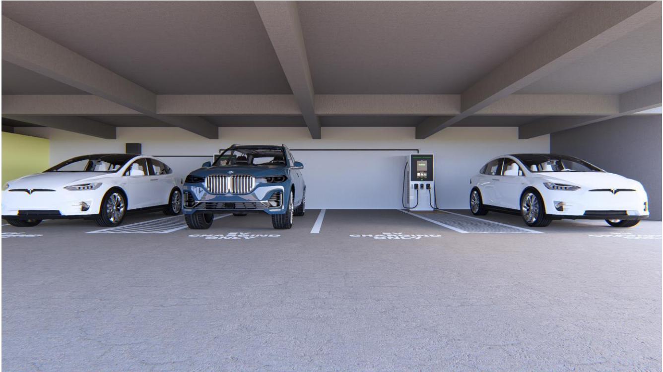
Figure 4-5: Dual-port charger layout with ADA-compliant stall configuration, including access aisle, directional markings, and charger placement optimized for forward entry and exit.
